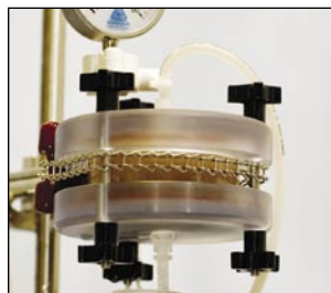
Figure 3a. This 50-cm 2 , 3-cm tall filter housing may be ordered from www.ertelsop.com (part # LAB 50P). Accessories are listed at the back of this document (Table 5).
